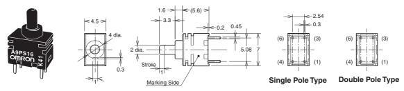
Note: NO.(4) and (6) terminals in the SPDT models are dummys to support the Switch case.
